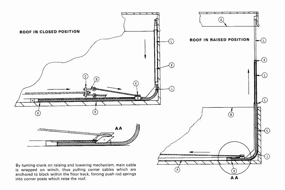
ROOF IN CLOSED POSITION: Position of flexible pushrod in the closed position is between X & X.
