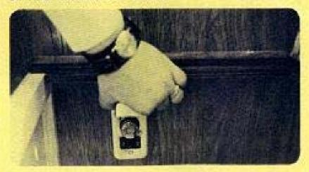
An extension cord will be necessary to connect to 110 volt power. Usually a 25 foot or longer cord is necessary. Use a number 16 3-wire cord.
